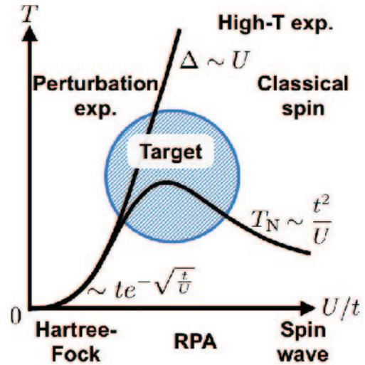
Fig. 1: Target region and valid approaches in the parameter space of interaction strength ( $U/t$ ) and temperature ( $T$ ).
