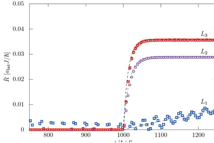
Fig. 1: Domain wall velocity as a function of time ( $t$ ). Staggered magnetic field is applied for  $t > 1000$ . The open squares are numerical results for a ferromagnet (blue) and collinear antiferromagnet (red). The open circles are those for  $\text{Mn}_3\text{Sn}$ . The dashed lines  $L_1$ ,  $L_2$ ,  $L_3$  are analytic solutions for FM,  $\text{Mn}_3\text{Sn}$ , and collinear AFM, respectively.
