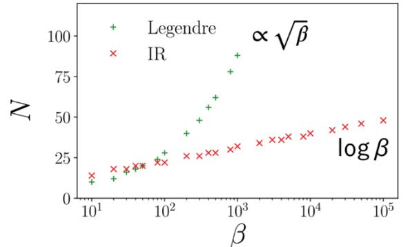
Fig.1: The number of expansion coefficients required to represent the Green's function.
